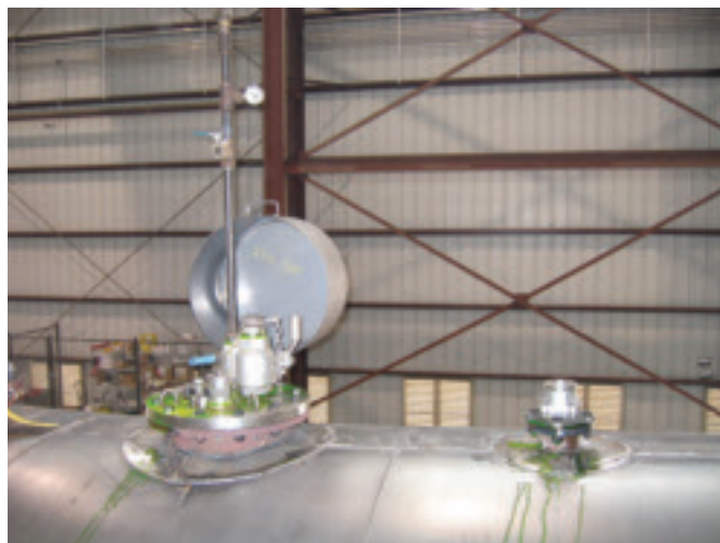
Fig. 6 — Once all the fittings have been attached, the inside of the car is checked for cleanliness, all openings are closed, and the car pressurized to determine there are no leaks at any of the fittings.
