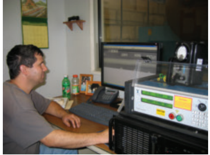
Fig. 4 — Inspector Spencer Scallan examines a CMOS image. The CMOS equipment is used to inspect the closure weld that joins the two tubs together to form a tank.
