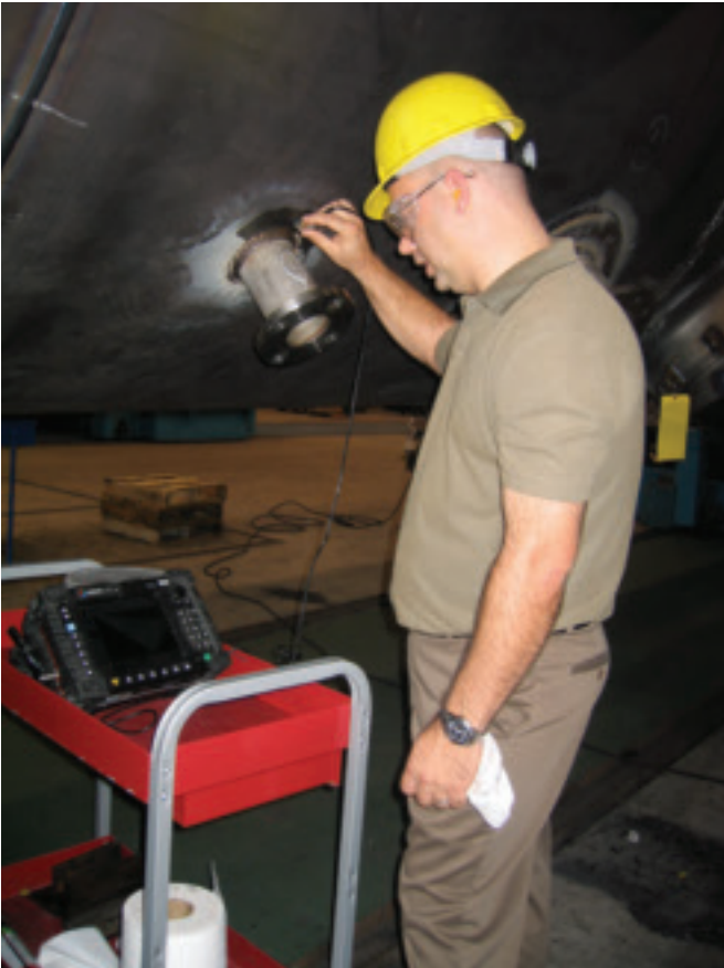
Fig. 5 — Kenneth Leblanc, an ASNT Level II Certified UT inspector and Level III inspector in radiography, checks the quality of a nozzle weld.
