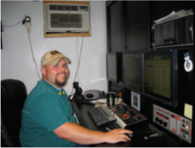
Fig. 3 — Inspector Jason Couvillion operates the fluoroscope and interprets the x-ray images. Porosity, slag, and incomplete fusion are the more common discontinuities he'll locate with the equipment.
